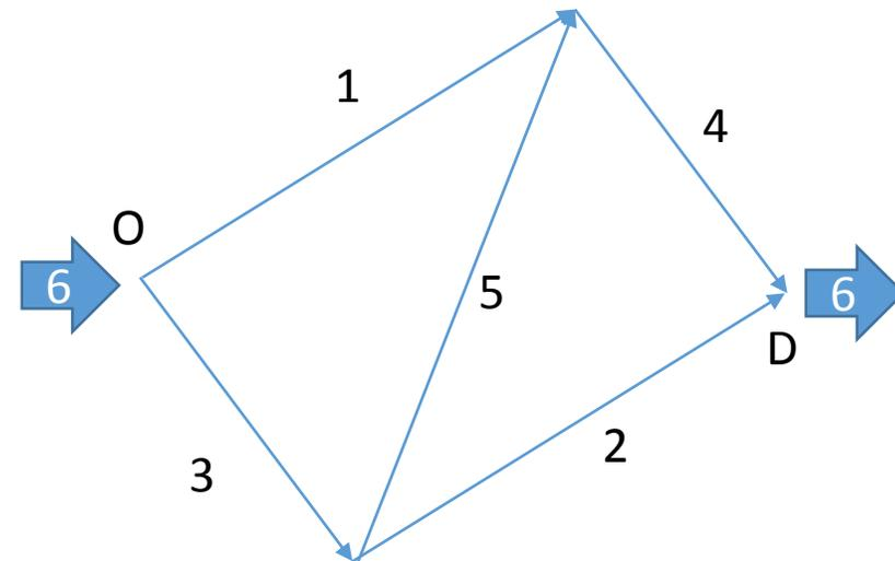
$$\begin{aligned} t_1[x_1] &= 50 + x_1 \\ t_2[x_2] &= 50 + x_2 \\ t_3[x_3] &= 10x_3 \\ t_3[x_4] &= 10x_4 \end{aligned}$$
