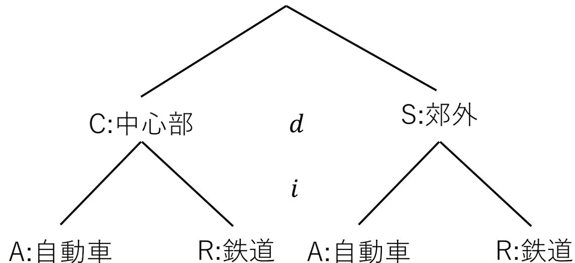
$$P(i|d) = \frac{\exp(\mu(V_i + V_{di}))}{\sum_{i'} \exp(\mu(V_{i'} + V_{di'}))}$$
